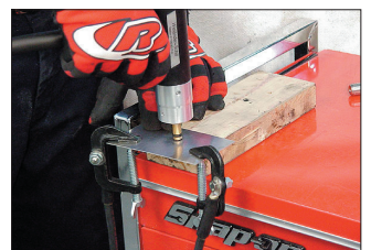
Figure 3—Perform a test stud weld on material of similar alloy and thickness as the panel on the vehicle that will be welded.
