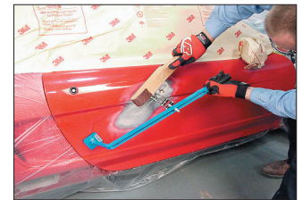
Figure 7-A steel rod, anchored by the washers, is pulled by a leverage bar to pull out the dent.
