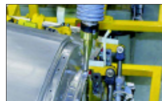
Figure 1—Mazda's new friction stir welder making a weld on a body assembly.
