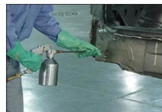
Figure 3—Anti-corrosion compound is applied to the inside of a rear rail using an extension wand.
