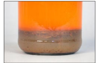
Figure 1—Sediments of contamination are evident in this sample of contaminated diesel fuel.
