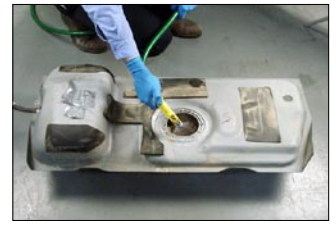
Figure 3—After draining, clean a contaminated fuel tank with water.
