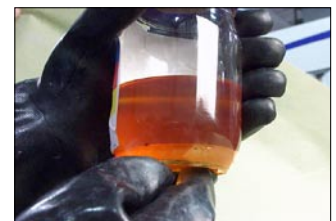
Figure 2—Drain gasoline into a clear jar to look for signs of contamination.
