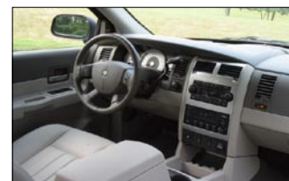
Figure 1—The driver airbag module protective trim cover with the chrome Dodge emblem may be removed from the airbag module and is available as a separate replacement part. (Courtesy of DaimlerChrysler)
