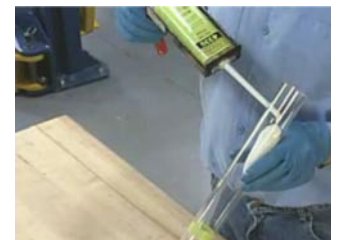
Movie—This video shows acoustical foam filler being applied too slowly.
