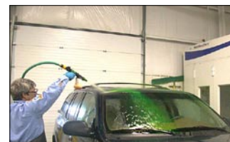
Figure 2—An air-boost flow is used to simulate harsh weather conditions.
