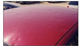
Figure 4—Horizontal panels like this roof skin receive the most damage from a hailstorm.
