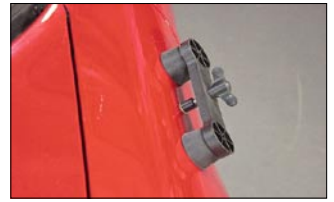
Figure 5—To remove damage with this removal tool, the wing-nut on the adhesively bonded stud pulls against the bridge that straddles the damage.
