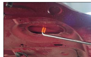
Figure 2—The plastic tip on this PDR tool will help avoid damaging the coatings on the panel backside.
