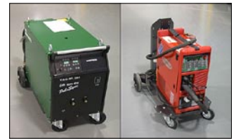
Figure 2—These welding machines provide pulse features that provide lower heat input.
