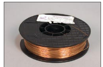
Figure 3—Copper-silicon (CuSi3) is the most common type of electrode wire used for MIG brazed joints.
