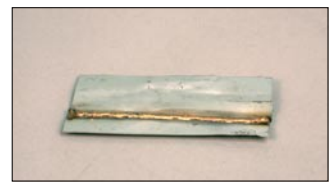
Figure 4—The bead of a MIG-brazed weld should not lay flat on the joint.
