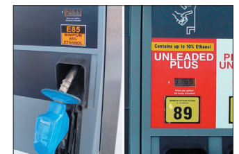
Figure 2 – Gas pump labels typically identify how much ethanol is in a fuel mixture.
