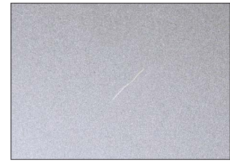
Figure 3— Small scratches may “disappear” in a self-healing clearcoat.
