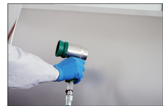
Figure 3– Hand-held air multipliers are one example of equipment that can be used to provide increased air movement to aid drying efficiency of waterborne materials.
