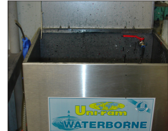
Figure 2– Cleaning a spray gun used to apply waterborne materials may require specific solutions (top) and equipment (bottom).
