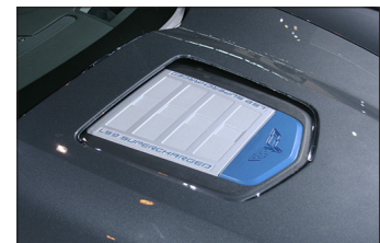
Figure 5— The carbon fiber hood on the ZR1 has a polycarbonate window to display the supercharger.
