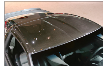
Figure 4— The exposed weave carbon fiber on the ZR1 has a special additive applied to protect against UV radiation.
