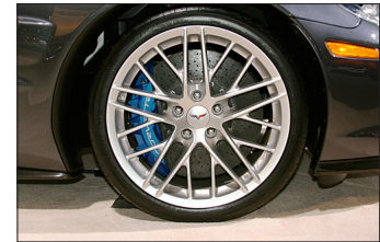
Figure 3— Carbon-ceramic brake rotors require ZR1-specific tools when servicing the wheels or brakes.
