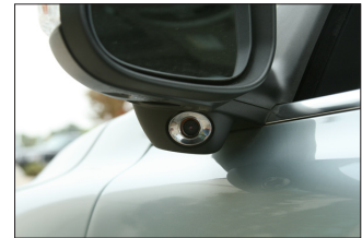
Figure 1– Volvo Blind Spot Information System (BLIS) cameras are located on the door mirrors.
