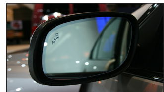
Figure 4– The 2010 Ford Taurus has visual indicators on the door mirrors to indicate the presence of an object in a blind spot.
