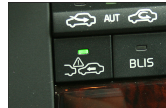
Figure 2– The Volvo BLIS may be switched on or off using the instrument panel switch.
