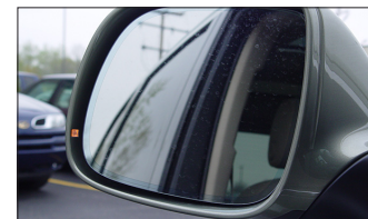
Figure 3– The Audi Q7 has yellow LED indicators on the door mirrors to indicate the presence of objects in the blind spot.
