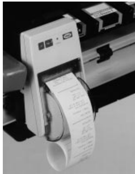
Figure 5—A printout of the headlight aiming dimensions is available with the system. (Courtesy of Hopkins Manufacturing Corporation)
