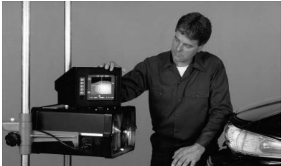
Headlight aiming can be as basic as aiming the lights at a screen, or as high tech as directing a laser beam to record a digital image of the headlight beam. (Courtesy of Hopkins Manufacturing Corporation)
