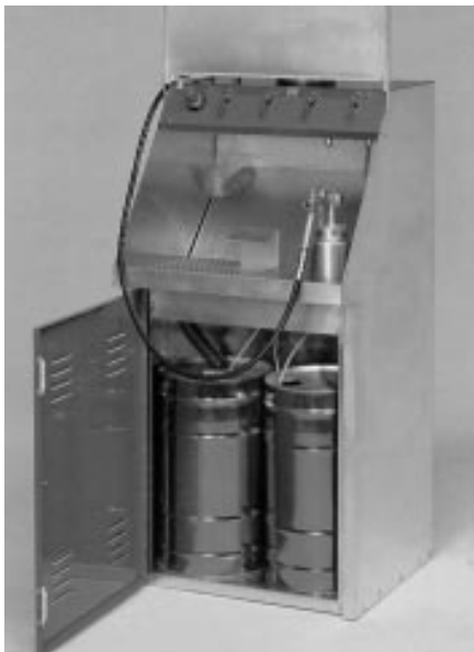
Figure 3—An enclosed gun cleaner, that recycles the cleaning solvents used, is a requirement in several regional VOC regulations. (Courtesy of Becca Recycling Technologies, Inc.)
