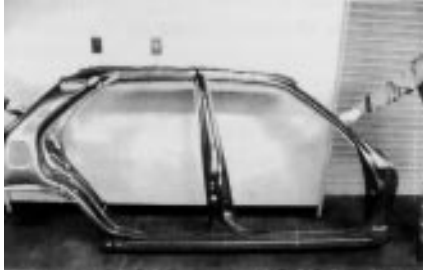
Figure 1—Sectioning is usually the best approach when repairing a side that has no factory seams. (Courtesy of Toyota)
